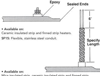
Mica insulated strip, ceramic insulated strip and finned strip heaters with leads.
